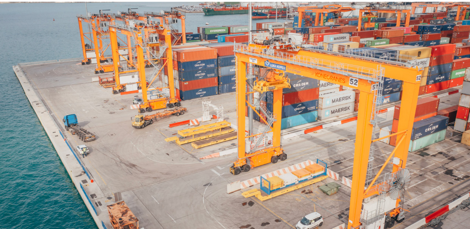
New e-RTG cranes, Photo: Kristjan Stojaković
