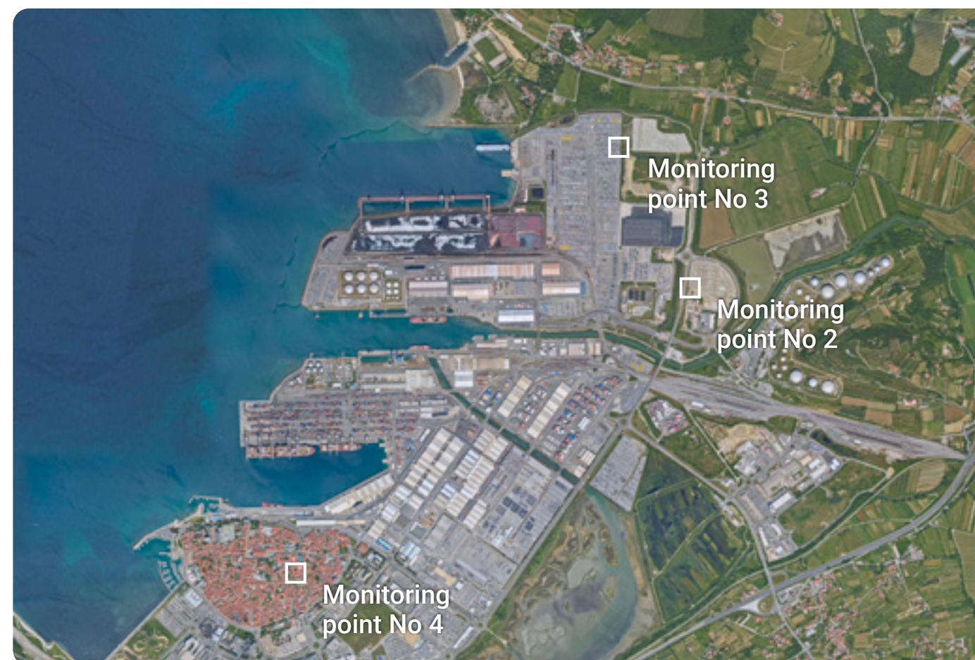
Locations of measuring devices for monitoring PM10 and PM2.5 dust particles
